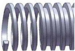
Single Start Screw - Lead & Pitch are the same
