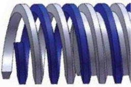
Double Start Screw - Lead is 2 X Pitch
