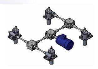
Our mitre boxes feature a compact design, which eliminates the need for an extended hub. With this design feature the bevel gear is supported by tapered roller bearings on both sides. The result is a higher horsepower rating, increased service-life, improved lubrication, and more flexible mounting compared to other brands.
