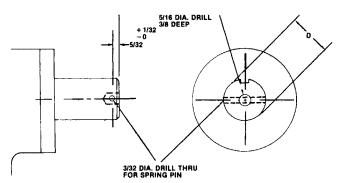
\*NOTE: SHIM OUT ON LIMIT SWITCH IF NECESSARY. WORM SHAFT END MUST NOT RUB SWITCH HOUSING.
